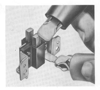
Place one terminal on the earthed carbon brush and the other on the brush holder plate.
