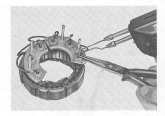
Solder the cable with a sufficiently powerful soldering iron (100 to 150 W), well heated, to ensure instant soldering.
